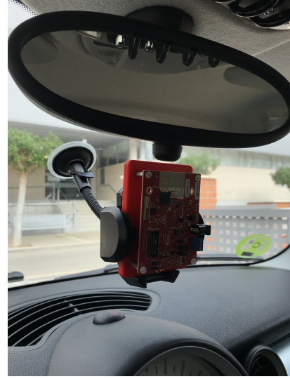
Fig. 4. Photograph of the radar attached to the front glass for testing.
